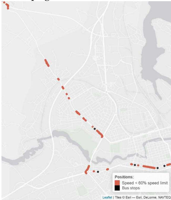
Figure 79 - Observations with low speed during morning peak in Norrköping.
