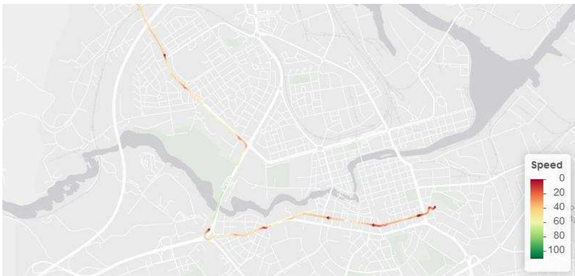
Figure 98 - The speed (km/h) of bus line 42 to Östra station 08:10 the 9 th of November, zoomed on Norrköping.
