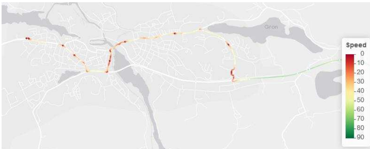
Figure 94 - The speed (km/h) of bus line 42 to Östra station 07:10 the 6th of November, zoomed on Finspång.
