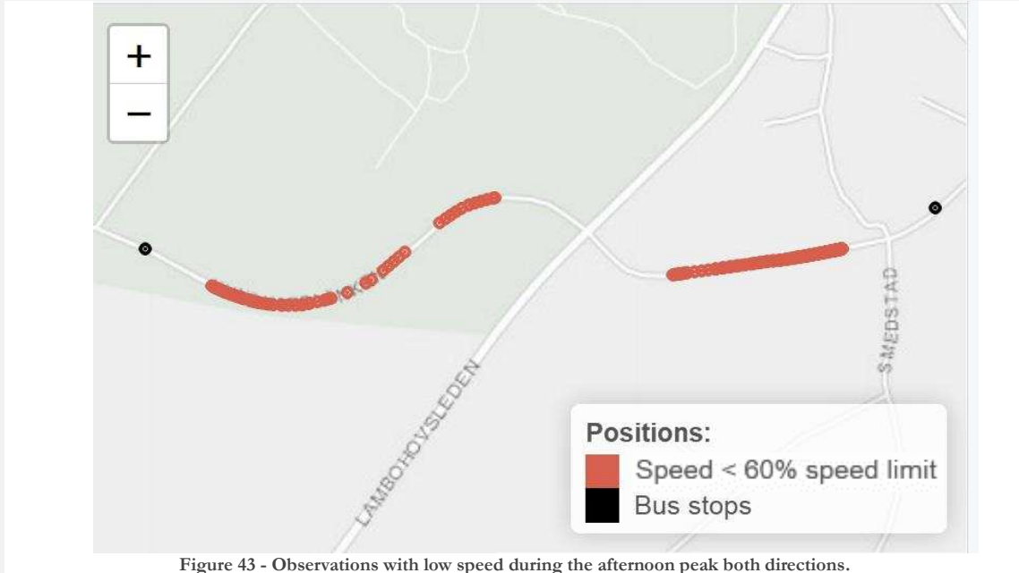
Figure 43 - Observations with low speed during the afternoon peak both directions.
