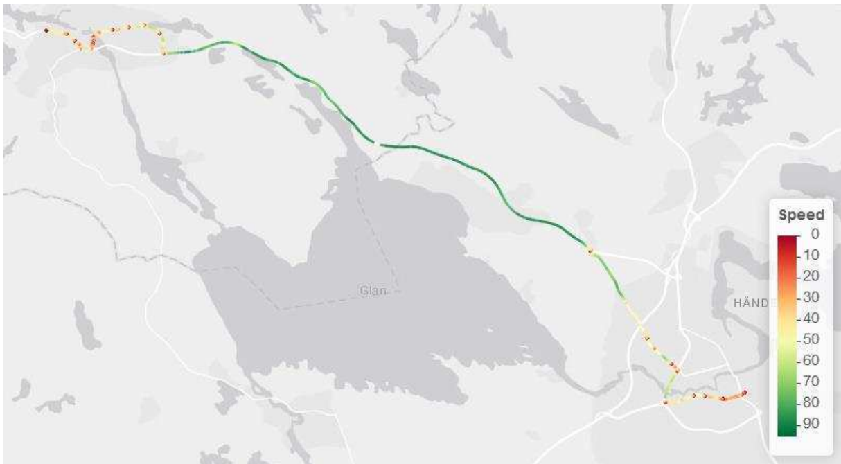
Figure 103 - The speed (km/h) of bus line 42 departure time 15:15 to Mellangrind at the 7 th of November.
